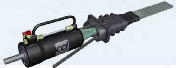
3. All stressing operations are controlled from the pump unit to ensure the operator's safety. The jack is extended and when the load is reached, the jack lock-off system is applied which firmly seats the wedge into the anchor head.
