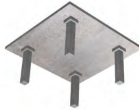
Solid flat slab with drop caps
